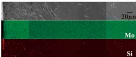
Fig. 2 Cross-sectional SEM image of the substrate with the corresponding EDS mapping of the MoSi 2 layer growth at 700 °C.
