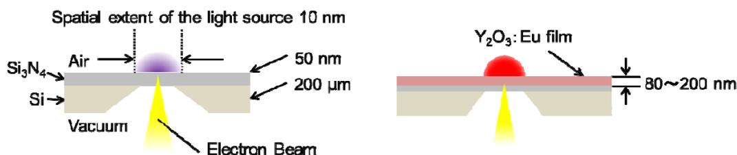
Figure 2 Schematics of luminescent thin films for EXA microscope.
