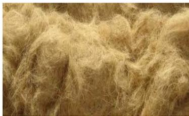
Fig. 1. Water Hyacinth fiber obtained by decortication to extract the fiber from stalk.
