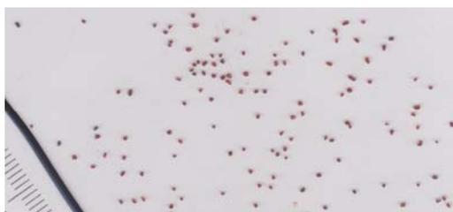
Fig. 2. An image scan of iron oxide-coated sand (IOCS). Millimeter marks are shown on the lower left.
