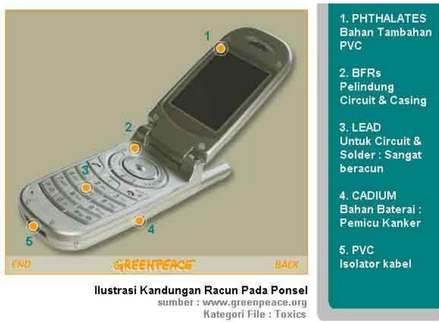
Figure 2. Illustration of harm component of a mobile phone
